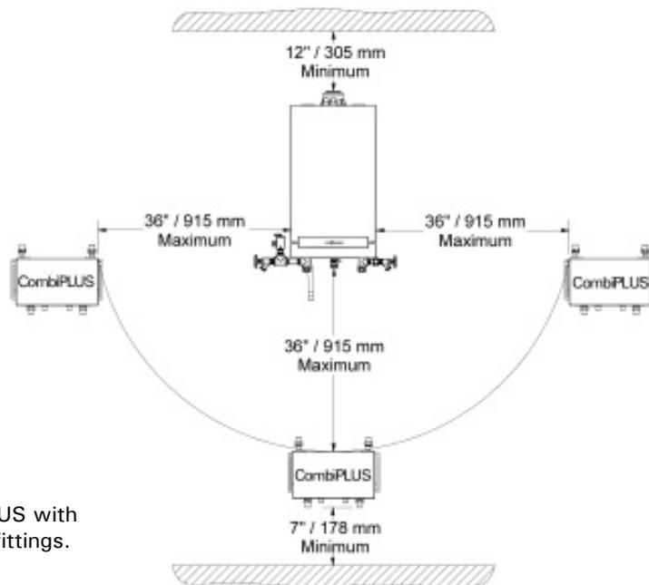
Shown is the maximum distance between the boiler and CombiPLUS using field supplied fittings and pipes.
