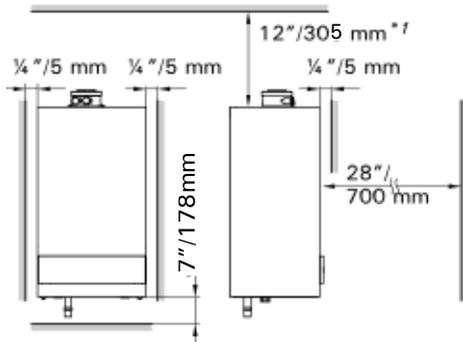
**Recommended minimum boiler and CombiPLUS Kit clearances to combustibles**
