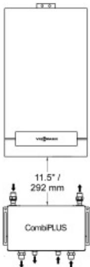
Min. distance between the boiler and CombiPLUS with Viessmann supplied 7" flex piping connection fittings.
