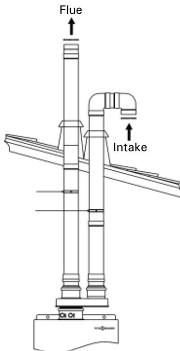
Two pipe system (room air independent) vertically vented
